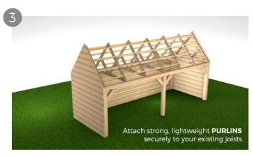
The minimum pitch needed for Tile Form Sheets is 12 degrees. If in doubt consult an engineer. The purlin spaces should be a maximum of 600mm apart. Please note, this is the recommended spacing and always seek advice from a structural engineer before installing.
