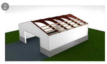
Sheets must be overlapped by a minimum of 600mm where the two Sheets meet. On a two-Sheet run remember to have a purlin under the overlap. These are guides and it depends on your roof's construction and pitch.
