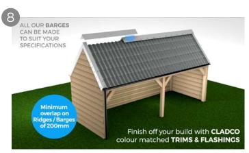
Ridge Flashings are used for the ridge on an apex roof, whereas for a single slope roof, you may need to use a Custom Flashing. To fit the Ridge, use Stitcher Screws through the Flashing and into the Sheets. Each Ridge should be overlapped by a minimum of 200mm.
