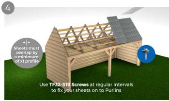
When installing Tile Form Sheeting you may need to lay the Sheets on the roof before fixing to ensure the overlap is sufficient. Sheets should be overlapped by a minimum of one profile when laid side by side. Sheets should be installed from right to left in a single Sheet run.
