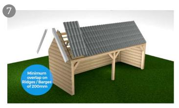
Once you have installed the final Sheet you can use Cladco Flashings for the sides and apex. Barges are used on the edges to help seal the building and provide an aesthetically pleasing effect. Please note, when joining or laying Flashings, there needs to be a minimum overlap of 200mm on Barges. Our 22mm Stitcher Screws are advised for securing Flashings in place.
