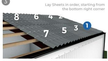
For a two-Sheet run, Sheets should be laid in a particular order starting at the eaves in the bottom right corner and then installing to the ridge. If the first Sheet is not laid perpendicular to the eaves and ridge, adjustments will have to be regularly made when laying other Sheets and a 'saw tooth' effect at the eaves will occur.
