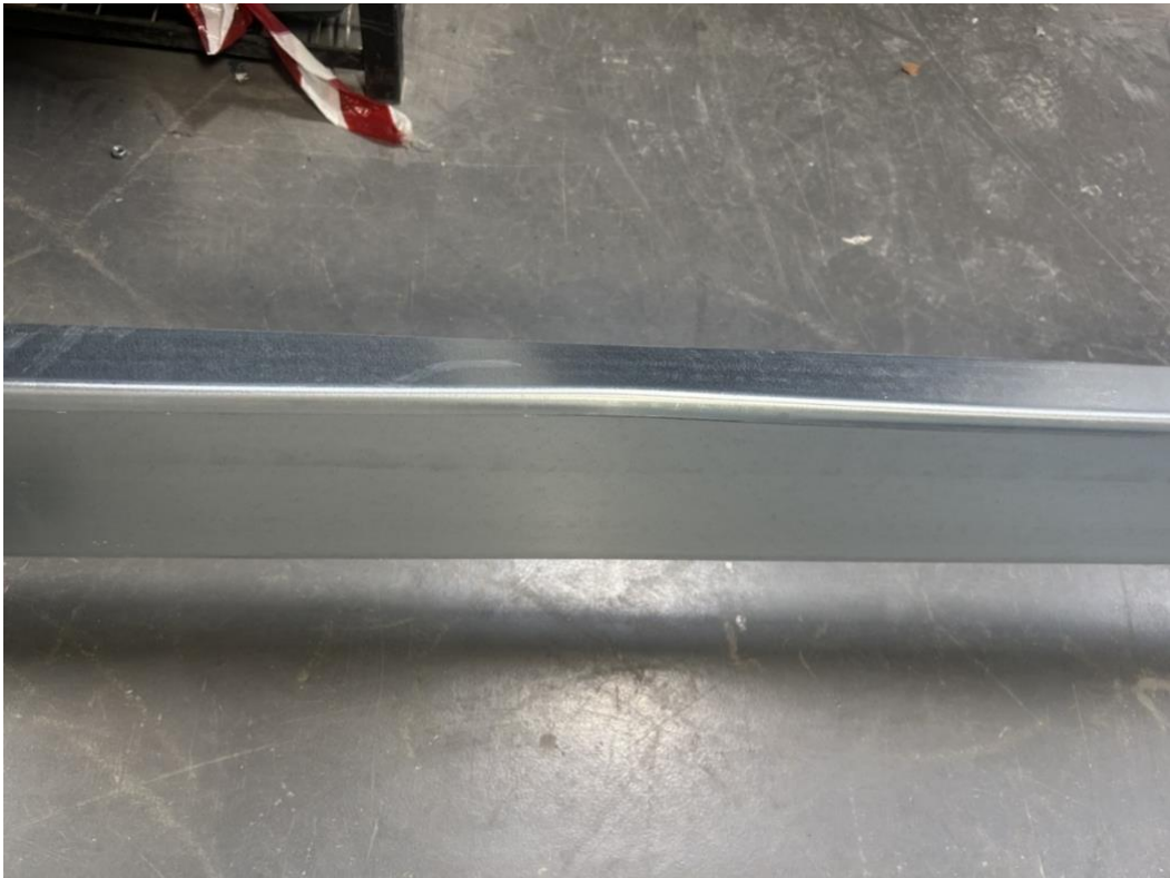
Figure 5 – Z Perlin Failure
