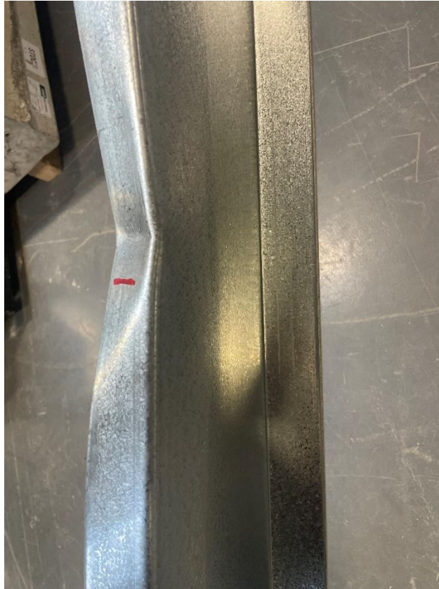
Figure 5 – Z Purlin Failure
