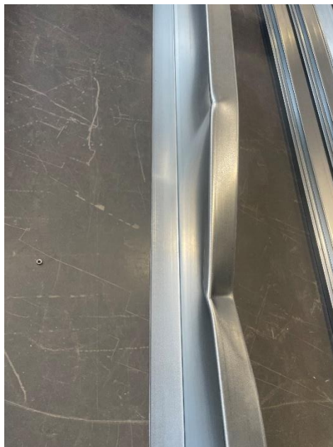
Figure 4 – Z Purlin Failure
