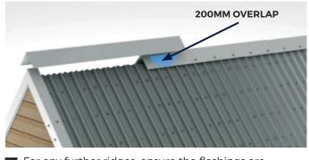
**Z** For any further ridges, ensure the flashings are O overlapped by a minimum of 200mm each time and install following the aforementioned process, With 22mm TEK stitcher screws inserted at the highest point of the profile at regular intervals. Any screw heads can then be capped with matching colour caps.
