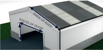
Measure the areas the Barges will be installed: the corners of the buildings, the edges of doors and the ends of the roof. Ensure to add an additional 200mm per Barge for overlaps. Barges are manufactured to 3m lengths.
