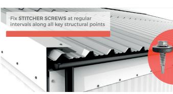
**Z** For any further Barges, ensure the flashings are overlapped by a minimum of 200mm each time and install following the aforementioned process, With 22mm TEK stitcher screws inserted at the highest point of the profile at regular intervals.
