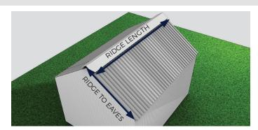
First, measure the length of your ridge, Ridges are manufactured at standard 3m lengths. When you are measuring the length of your ridge, be sure to add a minimum of 200mm per 3m to accommodate for overlapping ridge sheets. If the measurement of the ridge area does not equally divide into 3.2m sections, you can use additional overlap where required. This can be equal along the length for adequate coverage.
