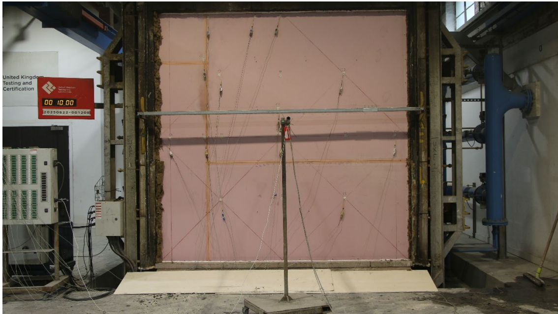
Figure 16 - The unexposed surface of the test construction after a test duration of 10 minutes
