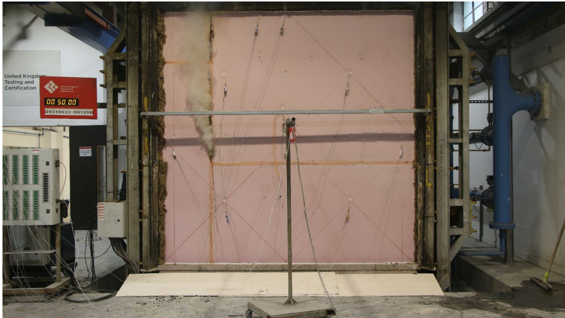
Figure 20 – The unexposed surface of the test construction after a test duration of 50 minutes
