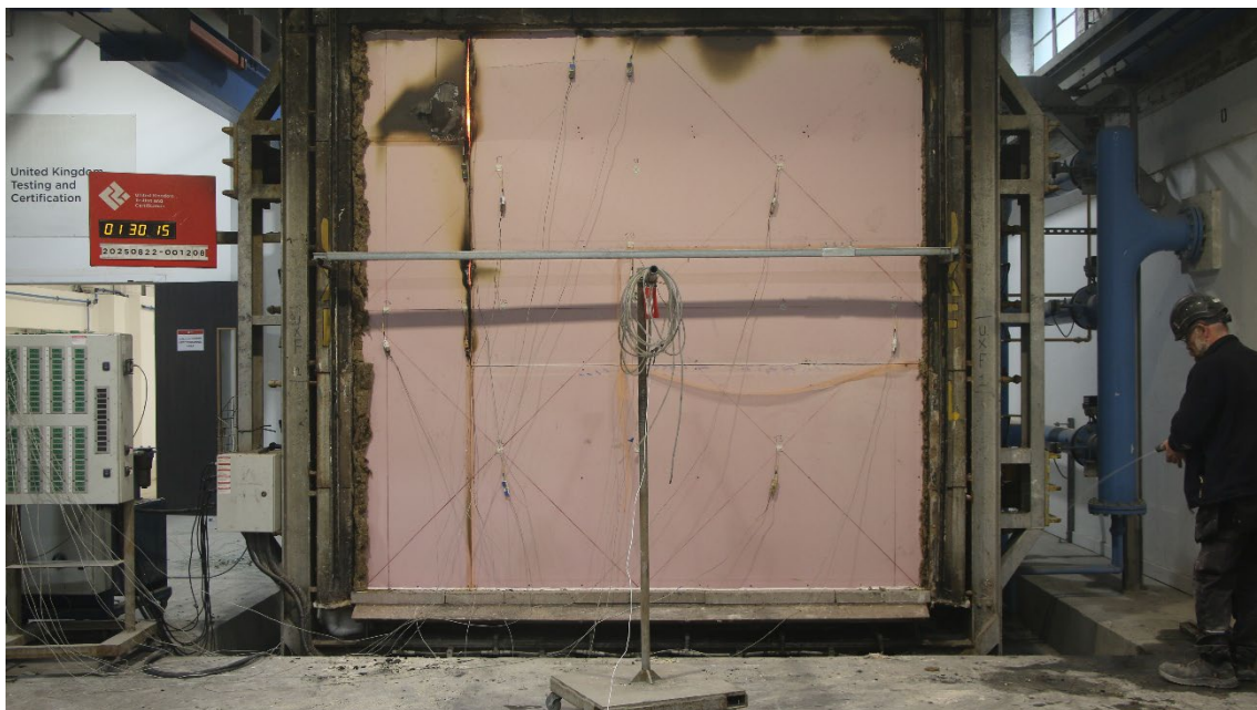
Figure 23 - The unexposed surface of the test construction after a test duration of 90 minutes
