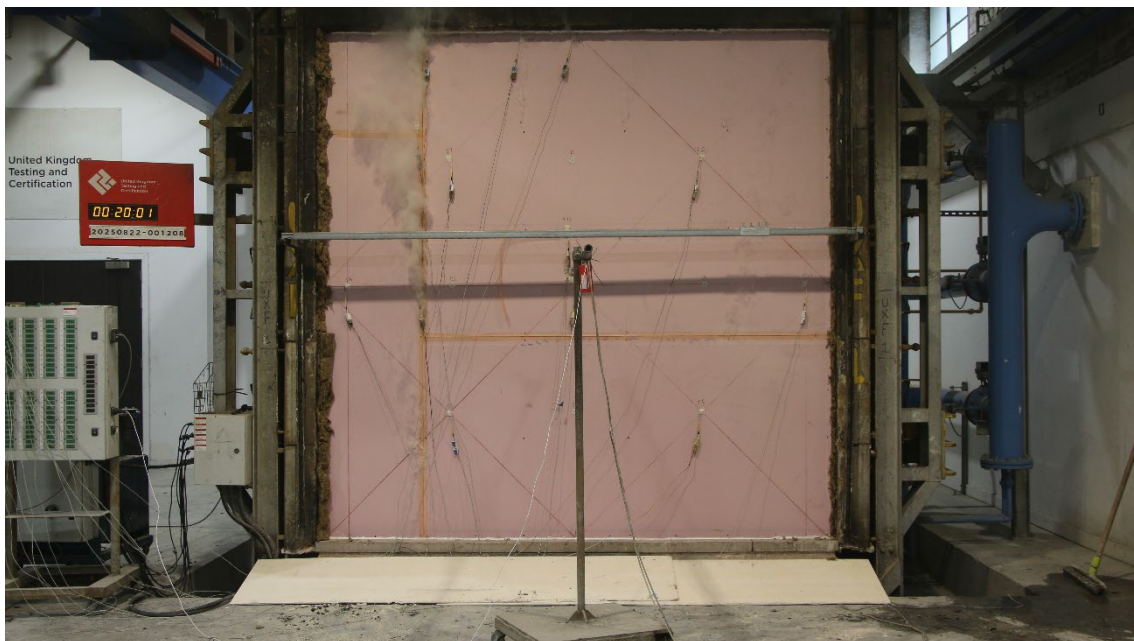
Figure 17 - The unexposed surface of the test construction after a test duration of 20 minutes
