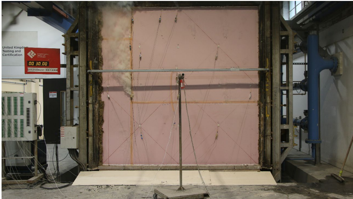
Figure 18 – The unexposed surface of the test construction after a test duration of 30 minutes
