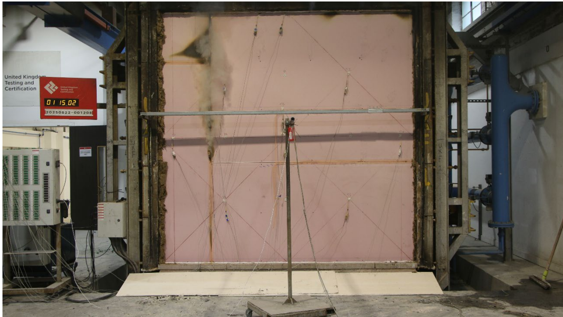
Figure 22 - The unexposed surface of the test construction after a test duration of 85 minutes
