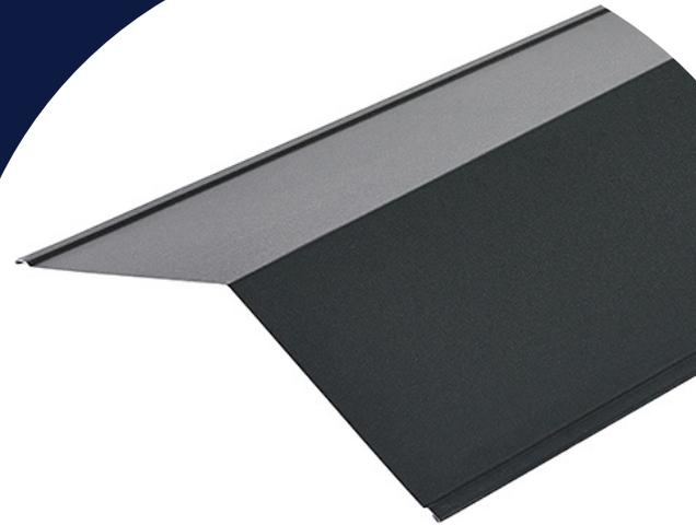
Ridge pieces are used at the apex of the roof to join the two sides together. Cladco Ridges are folded to a 130-degree internal angle and will flex 10 - 15 degrees either way, dependent on the angle of your roof. Ridges are a major component in any profiled clad apex roof and as they are available in a range of colours and finishes to match our roof sheets, they will enhance the aesthetics of any building.
