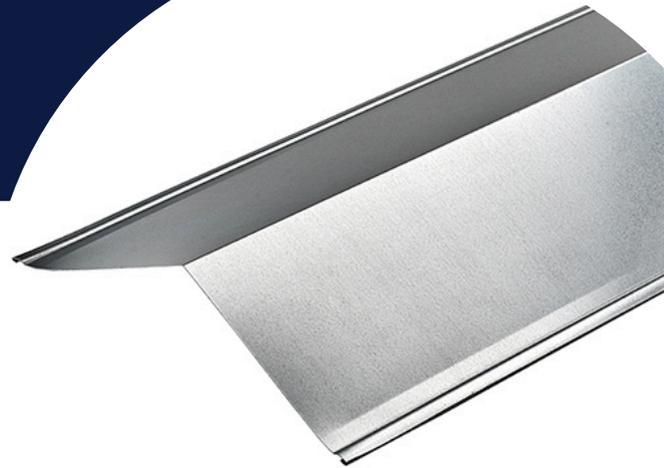
Ridge flashings are used at the apex of the roof to join the two sides together. At Cladco, our ridge flashings are folded to a 130-degree internal angle and will flex 10 – 15 degrees either way, dependent on the angle of your roof. Ridges are a major component in any profiled clad apex roof, and they will enhance the aesthetics of any building, especially in galvanised.
