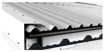
Foam fillers can be inserted underneath the eaves or the Ridges to further protect the building from weather conditions and prevent vermin from entering.
