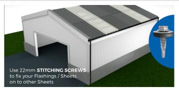
2 Begin by determining which end of your ridge is least affected by the wind. Your first ridge flashing should be laid at this point, and each flashing thereafter overlapped by the next flashing on the run by an absolute minimum of 150mm.
