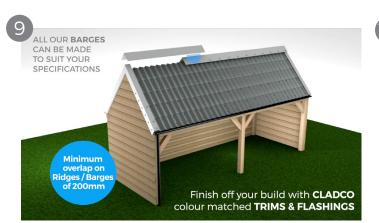
Ridge Flashings are used for the ridge on an Apex roof, where as for a single slope roof you may need to use a custom flashing. To fit the ridge use stitcher screws fix through the flashing and onto the rib/high point of the sheet. Lay ridge caps from the opposite end of the roof to the direction of prevailing winds. Each ridge should be overlapped by a minimum of 200mm.
