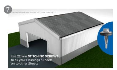
Barge flashings can be used to seal and finish off the ends of your roofing project. Flashings can ensure the building is watertight and prevent birds and water from entering the building. It is good practice to use silicone sealant/adhesive and stitcher screws to ensure a robust weather resistant join on side laps.
