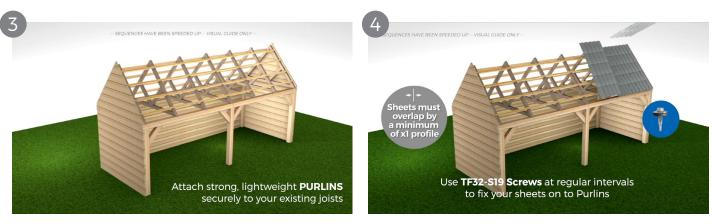
The minimum pitch needed for tile sheets is 12 degrees. If in doubt consult an engineer. Please note, these are recommended spacings but always seek advise from a structural engineer before installing. When installing the box profile sheeting you may wish to lay the sheets on the roof before fixing to ensure the overlap is sufficient. Sheets should be overlapped by a minimum of one tile profile when laid side by side.
