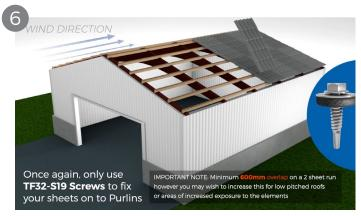
Sheets should be overlapped by the next sheet in the run by at least one tile profile ('side laps'). Adjacent runs of sheets should overlap each other by at least 600mm. Please note, we can only supply maximum length of 5 metres. If you require a longer length, its recommended to do a two sheet run.
