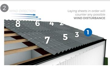
For a two sheet run, sheets should be laid in a particular order to the prevailing wind. Start at the eaves and in the corner away from the direction of the prevailing wind (this will help to prevent side laps facing into the wind and water ingress). If the first sheet is not laid perpendicular to the eaves and ridge, adjustments will have to be regularly made when laying other sheets and a 'saw tooth' effect at the eaves will be seen.
