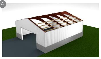
The minimum pitch needed for tile sheets is 12 degrees. On a two sheet run its imperative to have a purlin underneath the sheets overlap as shown in the image above. This can vary dependant on your roof construction and degree of pitch. The purlin spaces should be no more than 600mm apart, however always consult a professional prior to completing any work.
