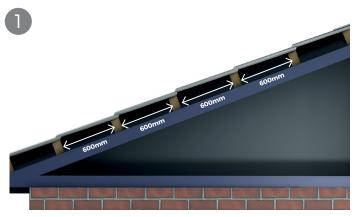
Purlin spaces for tile sheets need to be 600mm apart. These need to be in the correct place to be able to fix correctly at the top end of every second tile as shown.
