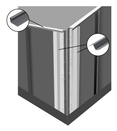
12 Measure and cut Z Bars to fit at the corner of a wall on either side. Install one Z Bar 90mm from the exterior edge. To better gauge its position, place a Corner Flashing section over the Bars and mark where the Z Bar will go on the adjoining wall.
