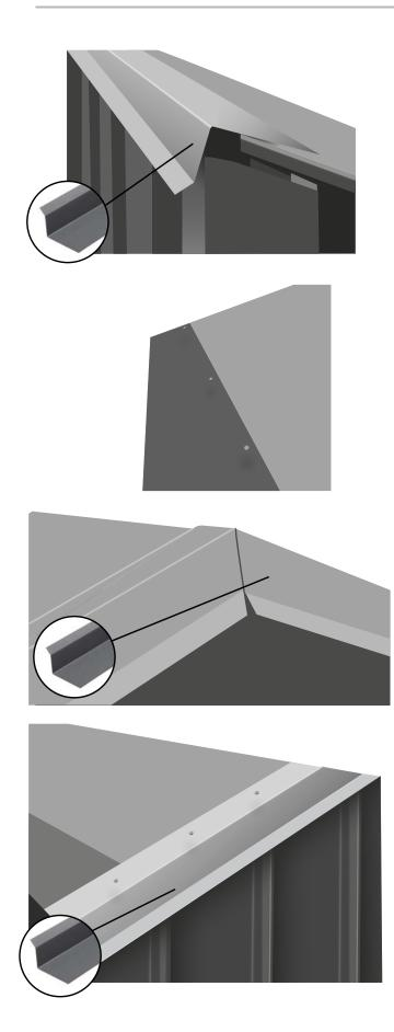
**1** If you are installing a mono-pitched roof, start by measuring and fixing Mono Ridge Backer Plates along the top edge of the roof using Annular Ring Nails. If you are installing a dual-pitched roof, move on to the next step.
