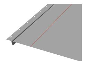
12 Repeat the previous step until you reach the final Sheet. Measure the width of the final Sheet and add 25mm for the Verge upstand. Cut off the fixing holes and fold the 25mm upstand along the left-hand side and top edge using hemming tools. The max width of this Sheet will be 470mm.
