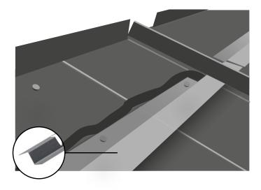
16 To install the Ridge Flashing, align the Z Bars (Notched) along the top of your roof. To help do this, temporarily place a Ridge Flashing or Mono Ridge piece over the apex and mark the position of the Z Bars. Use a string line and chalk mark to place Z Bars.
