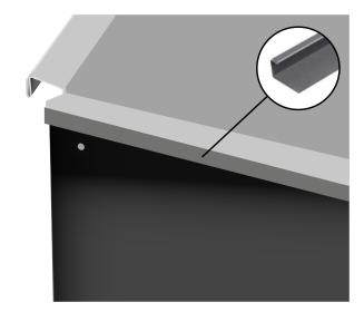
**10** Position and secure the Sheet over the seam using a rubber mallet to tap into place. Using Ring Nails, secure the left side of the last Sheet down the edges of the corner (one nail every 200mm).
