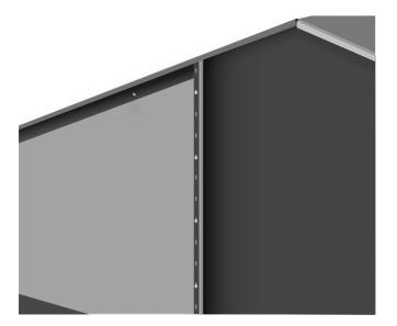
Continue to install Sheets to all walls and at gable ends, adjusting the angle of the cut edge according to the roof's pitch. Sheets can be centralised with the apex of the roof and fixed in place using Ring Nails every 3-4 fixing holes (every 200mm).
