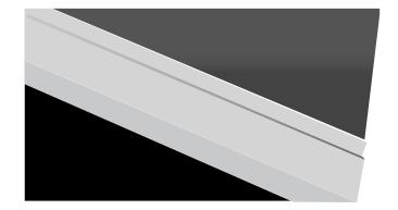
Tap the final Sheet at the base to nudge it into position over the Eaves Flashing and tap over the seam to secure it in place. Ensure Sheets are fully clipped together. The left-hand edge should align with the Verge Backer Plate.
