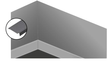
14 Measure and cut the Verge Flashing to length and install over the 25mm upstand and Backer Plate. For apex roofs, cut at an angle to sit flush with the adjoining Verge Flashing at the apex.
