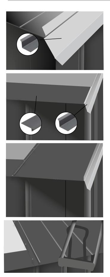
6 Working from right to left, measure the width of the first Standing Seam Sheet and include 25mm for the verge upstand. The maximum width of the first sheet will be 445mm after cutting off the seam.
