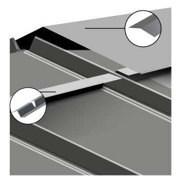
**18** Slide the Ridge Flashing over the Z Bars on both sides to fit into place. Secure the Flashing by clamping the edges using hand seaming pliers to fix the Flashing into place. For Mono Ridge Flashings, pull the Flashing over the Backer Plates and Z Bars and clamp into place.
