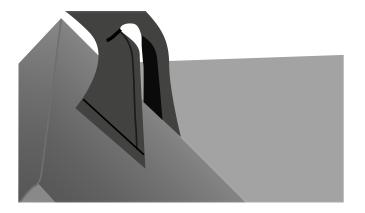
15 Using seaming pliers, clamp the bottom and top edges of the Verge Flashing around the Verge Backer Plate and upstand to create a tight seal. Finish each side of the roof with a Verge Flashing piece.
