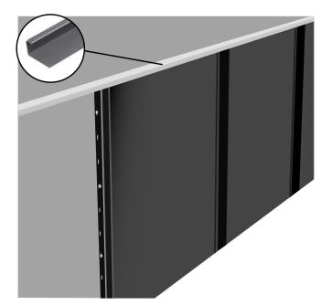
**9** Secure the Sheet in place using Ring Nails every 3-4 fixing holes (200mm). Continue securing the rest of the Cladding Sheets following the previous step until you get to the last Sheet. Measure the width of the final Sheet and cut it to size along the fixings side of the Sheet to complete the final run of Cladding along the wall.
