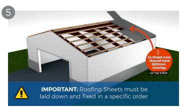
Sheets must be overlapped by a minimum of 600mm where the two sheets meet. Sheets should overlap side by side by at least one tile profile.
