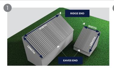
A single slope roof sometimes referred to as mono pitch or lean to roof. When working out your sheeting requirements, we require the length and width as shown in the diagram for us to be able to help you with a quotation. A width measurement is used to calculate the number of sheets required. The length measurement is used to calculate the length of sheets required.
