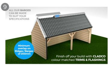
Ridge Flashings are used for the ridge on an Apex roof, where as for a single slope roof you may need to use a custom flashing. To fit the ridge use stitcher screws fix through the flashing and onto the rib/high point of the sheet. Lay ridge caps from the opposite end of the roof to the direction of prevailing winds. Each ridge should be overlapped by a minimum of 200mm.
