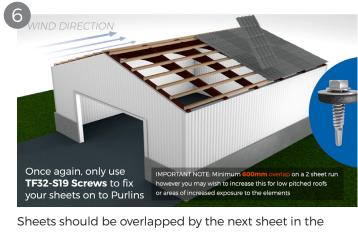
Sheets should be overlapped by the next sheet in the run by at least one tile profile ('side laps'). Adjacent runs of sheets should overlap each other by at least 600mm. Please note, we can only supply maximum length of 5 metres. If you require a longer length, its recommended to do a two sheet run.
