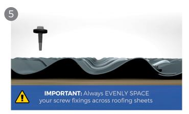
When fixing your tile sheeting its imperative they are fixed at the valley, we recommend using TF32-S19 screws which are self drilling and self sealing. Please see image above.
