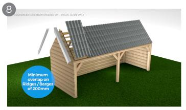
Once you have installed the final sheet you can use Cladco flashings for the sides and apex. Barges are used on the egdes to help seal the building and provide an aesthetically pleasing affect. Please note when joining / laying these there is a minimum overlap of 200mm on barges. Stitcher screws at 22mm are advised for securing flashings in place.
