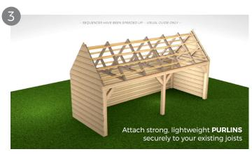
The minimum pitch needed for tile sheets is 12 degrees. If in doubt consult an engineer. Please note, these are recommended spacings but always seek advise from a structural engineer before installing.
