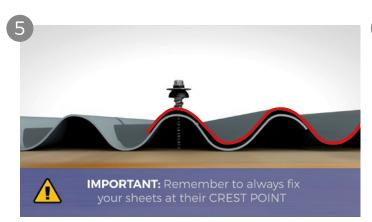
When fixing your corrugated sheeting its imperative they are fixed at the crest point, we recommend using 65mm BAZ screws which are self drilling and self sealing. Please see image above.
