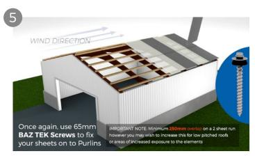
Sheets should be overlapped by the next sheet in the run by at least two profile or corrugations ('side laps'). Adjacent runs of sheets should overlap each other by at least 250mm ('end laps'). Please note, we can only supply a maximum of 6 metres. If you require a longer length, its recommended to do a two sheet run.
