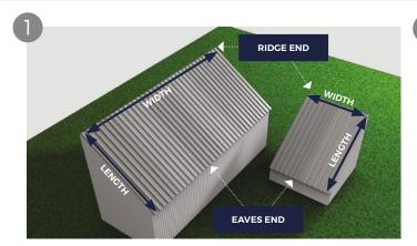
A single slope roof sometimes referred to as mono pitch or lean to roof. When working out your sheeting requirements, we require the length and width as shown in the diagram for us to be able to help you with a quotation. A width measurement is used to calculate the number of sheets required. The length measurement is used to calculate the length of sheets required.
