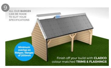
Ridge Flashings are used for the ridge on an Apex roof, where as for a single slope roof you may need to use a custom flashing. To fit the ridge use stitcher screws fix into the flashing and onto the rib/raised profile of the sheets. Lay ridge caps from the opposite end of the roof to the direction of prevailing winds. Each ridge should be overlapped by a minimum of 200mm.
