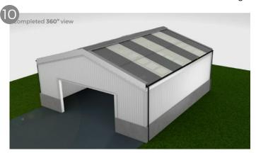
Finish your project by installing the ridge flashing along the centre where two sheets meet. You can then install guttering or fascia as required.
