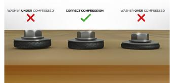
Do not over-tighten or under-tighten your screws as this can affect the performance of the washer and prevent it from sealing correctly. See diagram above.
