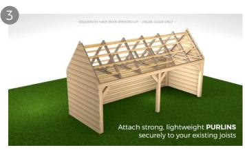
The minimum pitch needed for corrugated sheets is 10 degrees. If in doubt consult an engineer. The purlin spaces on average should be approximately 1.2m apart, however if using 0.5mm for the roof (which is normally used for side sheeting) you would need to reduce purlin spaces to no more than 1m apart. Please note, these are recommended spacings but always seek advice from a structural engineer before installing.
