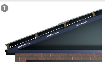
The minimum pitch needed for corrugated sheets is 10 degrees. On a two sheet run its imperative to have a purlin underneath the sheets overlap as shown in the image above. This can vary dependent on your roof construction and degree of pitch. The purlin spaces should be no more than 1.2m apart, however always consult a professional prior to completing any work.
