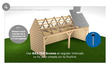
When installing the corrugated sheeting you may wish to lay the sheets on the roof before fixing to ensure the overlap is sufficient. Sheets should be overlapped by a minimum of two corrugations when laid side by side. Colour caps can be used to cover the silver screw head and matched to the roofing sheet colour.
