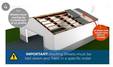
Sheets must be overlapped by a minimum of 250mm where the two sheets meet. Roof lights can be installed between the sheets but must have sheets either side for support. Sheets should overlap side by side by at least two corrugations.
