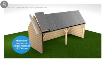
Once you have installed the final sheet you can use Cladco flashings for the sides and apex. Barges are used on the edges to help seal the building and provide an aesthetically pleasing affect. Please note when joining / laying these there is a minimum overlap of 200mm on barges. Stitcher screws at 22mm are advised for securing flashings in place.
