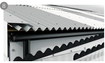
Fillers can help ensure a robust weather resistant seal, to prevent birds and vermin as well as water from entering the building. An eaves filler strip is designed to go under a sheet, while an opposite ridge filler strip is designed to go over a sheet. All foam filler strips should be bonded to the pans or valleys of the sheeting with a flexible, waterproof silicone sealant and should be continuous over the entire width of the sheeting.
