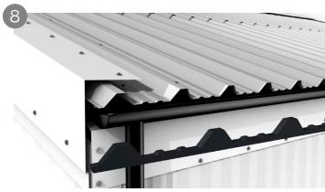
Fillers can help ensure a robust weather resistant seal, to prevent birds and vermin as well as water from entering the building. An eaves filler strip is designed to go under a sheet, while an opposite ridge filler strip is designed to go over a sheet. All foam filler strips should be bonded to the pans or valleys of the sheeting with a flexible, waterproof silicone sealant and should be continuous over the entire width of the sheeting.
