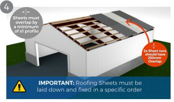
Sheets must be overlapped by a minimum of 250mm where the two sheets meet. Roof lights can be installed between the sheets but must have sheets either side for support. Sheets should overlap side by side by at least one profile.
