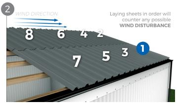
For a two sheet run, sheets should be laid in a particular order to the prevailing wins. Start at the eaves and in the corner away from the direction of the prevailing wind (this will help to prevent side laps facing into the wind and water ingress). If the first sheet is not laid perpendicular to the eaves and ridge, adjustments will have to be regularly made when laying other sheets and a 'saw tooth' effect at the eaves will be seen.
