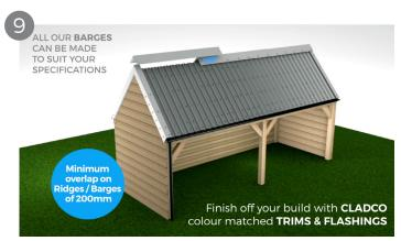
Ridge Flashings are used for the ridge on an Apex roof, where as for a single slope roof you may need to use a Custom Flashing. To fit the ridge use stitcher screws into the flashing and onto the sheets. Lay ridge caps from the opposite end of the roof to the direction of prevailing winds. Each ridge should be overlapped by a minimum of 200mm.
