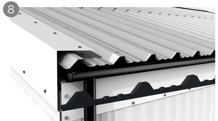
Fillers can help ensure a robust weather resistant seal, to prevent birds and vermin as well as water from entering the building. An eaves filler strip is designed to go under a sheet, while an opposite ridge filler strip is designed to go over a sheet. All foam filler strips should be bonded to the pans or valleys of the sheeting with a flexible, waterproof silicone sealant and should be continuous over the entire width of the sheeting.
