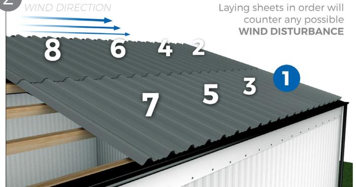
For a two sheet run, sheets should be laid in a particular order to the prevailing wins. Start at the eaves and in the corner away from the direction of the prevailing wind (this will help to prevent side laps facing into the wind and water ingress). If the first sheet is not laid perpendicular to the eaves and ridge, adjustments will have to be regularly made when laying other sheets and a 'saw tooth' effect at the eaves will be seen.
