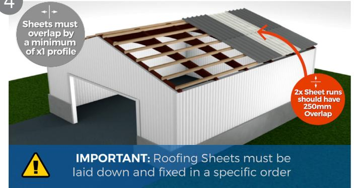
Sheets must be overlapped by a minimum of 250mm where the two sheets meet. Roof lights can be installed between the sheets but must have sheets either side for support. Sheets should overlap side by side by at least one profile.
