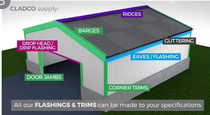
Custom Flashings can be made for projects to match the steel sheeting we offer. Flashings can provide weatherproofing to the building particularly at the ridge where two sheets meet.
