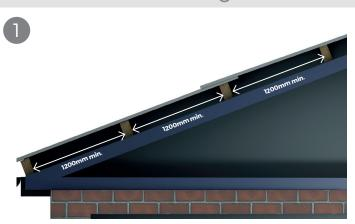
The minimum pitch needed for box profile sheet is 4 degrees. On a two sheet run remember to have a purlin under the overlap as shown. These are guides and it depends on your roof construction and pitch. If in doubt consult an engineer. Purlin spaces using 7 thickness sheet should be approximately 1.2m apart. Purlin spaces using 5 thickness sheet should be approximately 1m apart.
