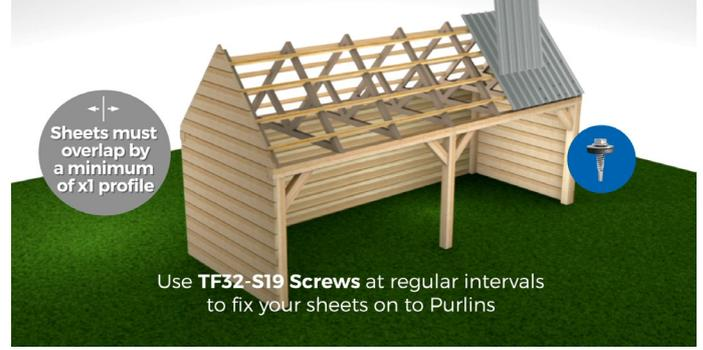
When installing the box profile sheeting you may wish to lay the sheets on the roof before fixing to ensure the overlap is sufficient. Sheets should be overlapped by a minimum of one box profile when laid side by side. Colour caps can be used to cover the silver screw head and matched to the roofing sheet colour.
