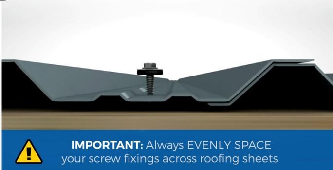
When fixing your box profile sheeting it's imperative they are fixed at the cvalley point, we recommend using TF32-S19 screws which are self drilling and self sealing. Please see image above.
