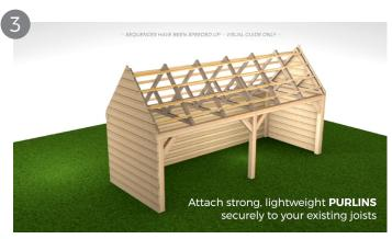
The minimum pitch needed for box profile sheet are 4 degrees. If in doubt consult an engineer. The purlin spaces on average should be a maximum of 1.2m apart, however if using 0.5mm for the roof (which is normally used for side sheeting) you would need to reduce purlin spaces to no more than 1m apart. Please note, these are recommended spacings but always seek advise from a structural engineer before installing.
