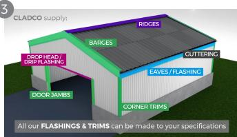
Custom Flashings can be made for projects to match the steel sheeting we offer. Flashings can provide weatherproofing to the building particularly at the ridge where two sheets meet.
