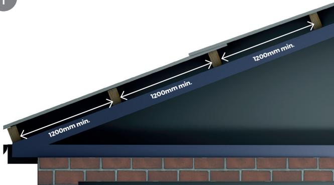
The minimum pitch needed for box profile sheet is 4 degrees. On a two sheet run remember to have a purlin under the overlap as shown. These are guides and it depends on your roof construction and pitch. If in doubt consult an engineer. Purlin spaces using 7 thickness sheet should be approximately 1.2m apart. Purlin spaces using 5 thickness sheet should be approximately 1m apart.
