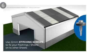
Barge flashings can be used to seal and finish off the ends of your roofing project. Flashings can ensure the building is watertight and prevent birds and water from entering the building. It is good practice to use mastic lapping tape and stitching screws to ensure a robust weather resistant joint on side laps.
