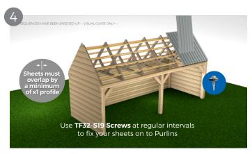
When installing the box profile sheeting you may wish to lay the sheets on the roof before fixing to ensure the overlap is sufficient. Sheets should be overlapped by a minimum of one box profile when laid side by side. Colour caps can be used to cover the silver screw head and matched to the roofing sheet colour.
