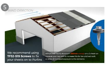
Sheets should be overlapped by the next sheet in the run by at least one profile ('side laps'). Adjacent runs of sheets should overlap each other by at least 250mm ('end laps'). Please note, we can only supply a maximum of 9 metres. If you require a longer length, its recommended to do a two sheet run.
