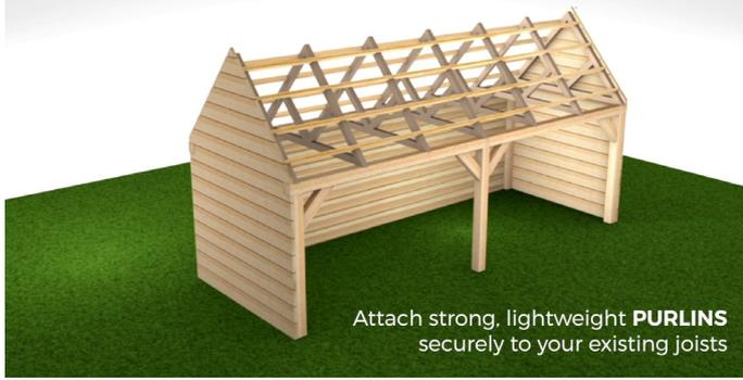
The minimum pitch needed for box profile sheet are 4 degrees. If in doubt consult an engineer. The purlin spaces on average should be a maximum of 1.2m apart, however if using 0.5mm for the roof (which is normally used for side sheeting) you would need to reduce purlin spaces to no more than 1m apart. Please note, these are recommended spacings but always seek advise from a structural engineer before installing.
