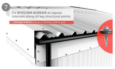
Stitcher screws are recommended to secure flashings. Screws should be no more than 400mm apart when securing the flashing. Colour caps can be used to conseal the top of the screw head.
