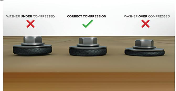
**TOP TIP** Do not over-tighten or under-tighten your screws as this can affect the performance of the washer and prevent it from sealing correctly. See diagram above.
