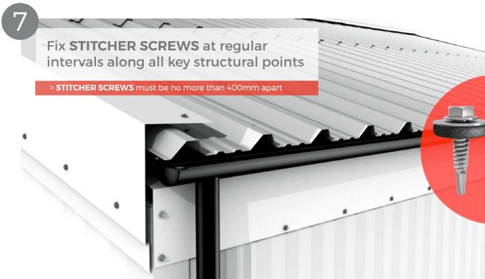
Stitcher screws are recommended to secure flashings. Screws should be no more than 400mm apart when securing the flashing. Colour caps can be used to conceal the top of the screw head.
