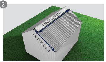
Apex roofs are separated by a central ridge. As per the diagram we require the length of sheet from ridge to eaves and the ridge length to calculate your requirements. You will need to measure both sides of the roof as the building/roof can vary in size from side to side. If the apex is uneven ridge to eaves will need to be taken on both sides.
