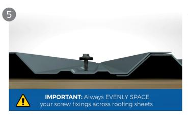
When fixing your box profile sheeting it's imperative they are fixed at the cvalley point, we recommend using TF32-S19 screws which are self drilling and self sealing. Please see image above.
