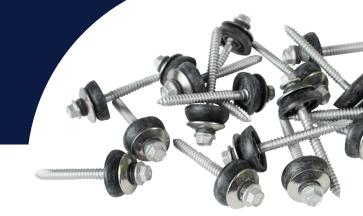
Cladco TEK type, self-tapping 65mm Screws to Wood are designed to fix Steel Corrugated Profiled Sheeting to Timber Purlins through the highest part of the Profile.
