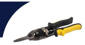
Straight Cut Tin Snips are designed to cut your Cladco Flashings and Roofing Sheets. With a hardened blade and serrated edges, they will cut through steel easily leaving a clean cut. Features include slip-resistant hand grips and lock and slip guards.
