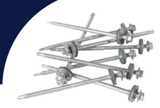
TEK Screws with a self-drilling fix are designed for fixing Sheets to light steel. TEK Screws are manufactured with a 5/16 inch hexagonal head and a 19mm bonded sealing washer to ensure they are watertight and secure.
