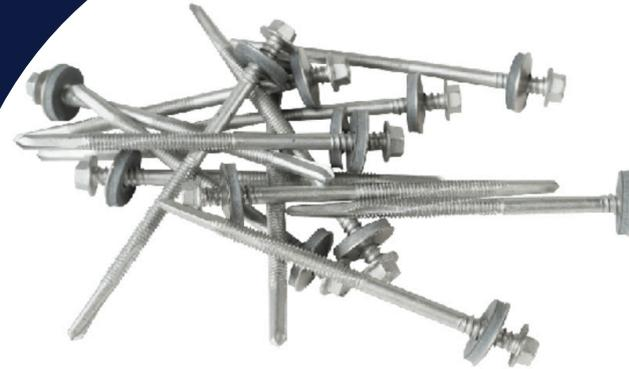
Cladco TEK Screws are self-drilling and designed for fixing Sheets to heavy steel. The TEK Screws have a 5/16 inch hexagonal head with 19mm bonded sealing washer to ensure they are watertight and secure.
