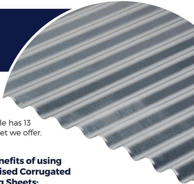
The most traditional looking roof sheets, the 0.7mm thickness of the Cladco Profiles galvanised corrugated roofing sheets provide the same aesthetic as 13/3 corrugated iron cladding profiles. With a width coverage 990mm when lapped, this profile has 13 corrugations of 3-inch round, the 0.7mm is the thickest 13/3 sheet we offer.
