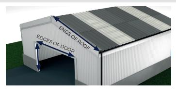
Measure the areas where the Barges will be installed: the corners of the buildings, the edges of doors and the ends of the roof. Ensure to add an additional 200mm per Barge for overlaps. Barges are manufactured to 3m lengths.
