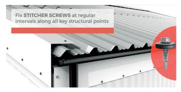
To rany further Barges, ensure the flashings are overlapped by a minimum of 200mm each time and install following the aforementioned process, using 22mm TEK stitcher screws inserted at the highest point of the profile at regular intervals.
